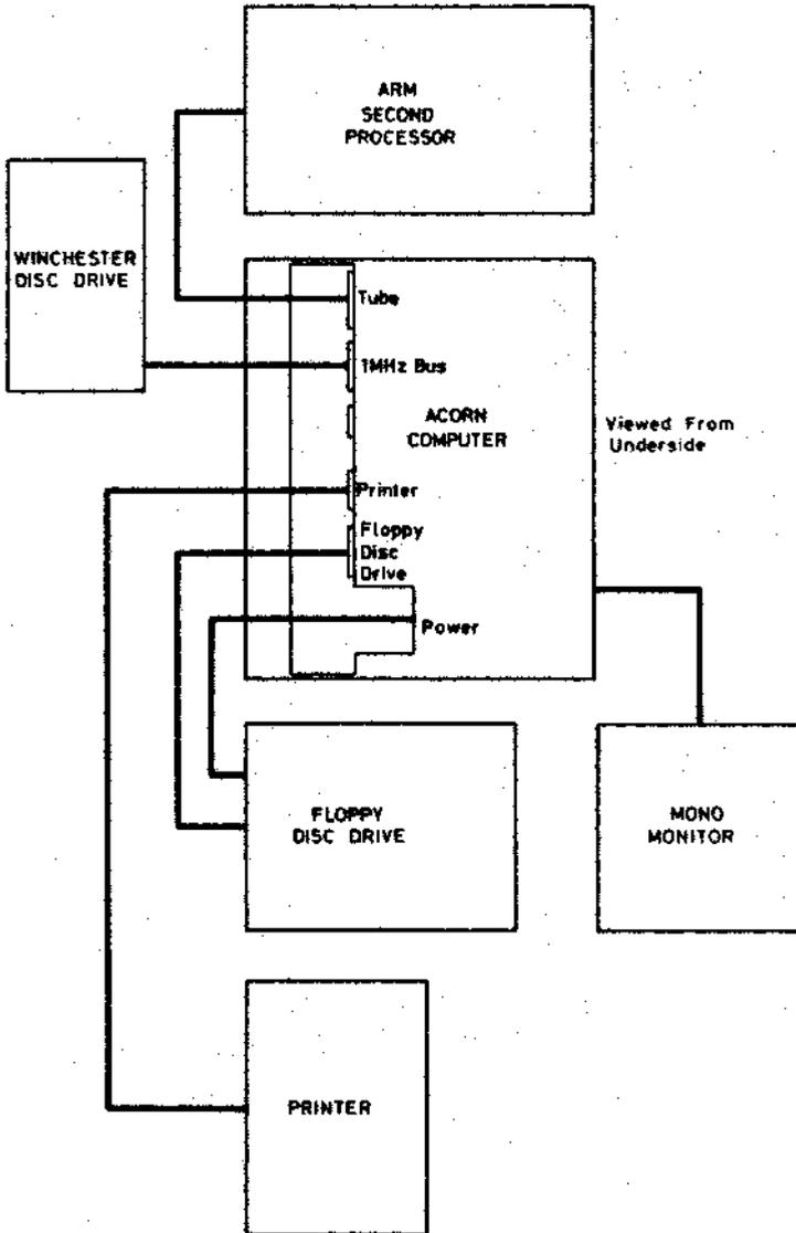
The cable supplied with the co-processor is captive at the co-processor end and has a 40-way IDC connector at the other end which plugs into the interface, under the BBC Model B or BBC Master microcomputer, marked TUBE. The co-processor has a separate mains lead for connection to a 240 V 50 Hz mains supply.
